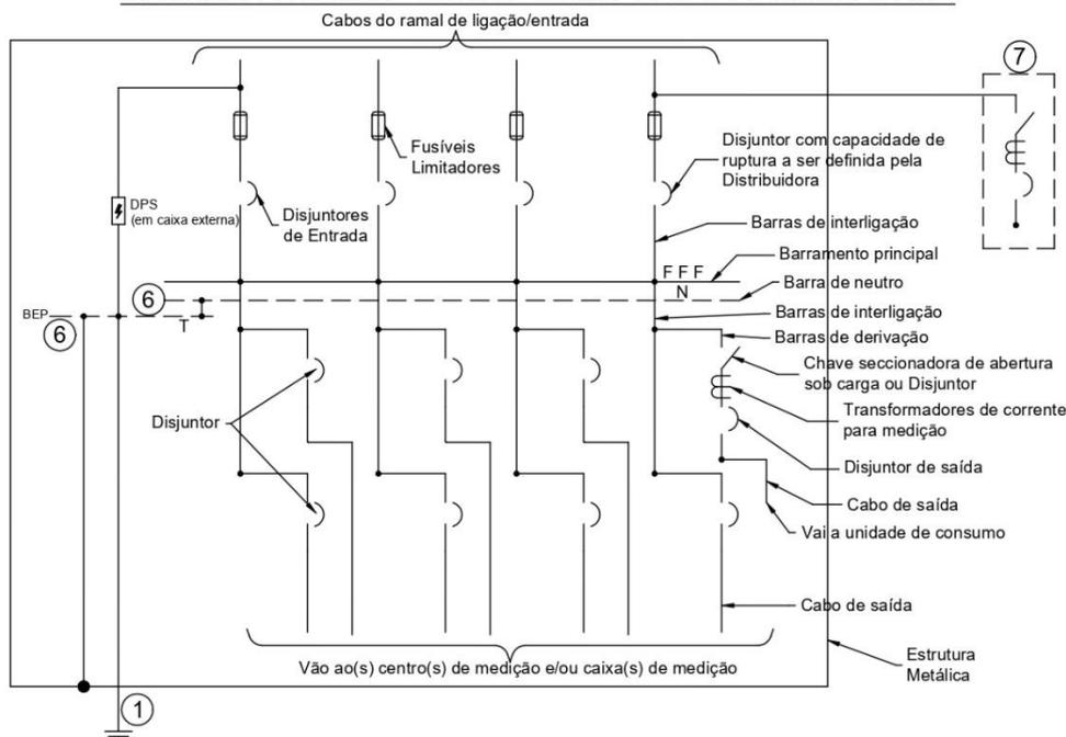
**DIAGRAMA UNIFILAR - TENSÃO 220/380 VOLTS**
